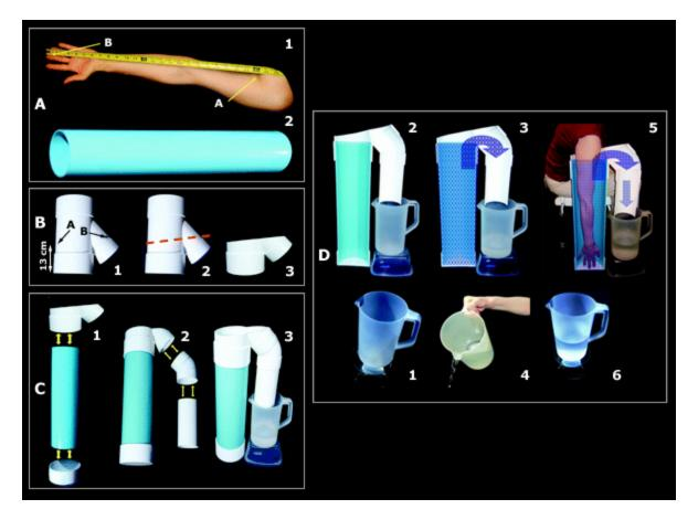
(A, B) Preparation of parts, (C) assembly, and (D) arm volume measurement procedure, including a longitudinal cross-section view.
